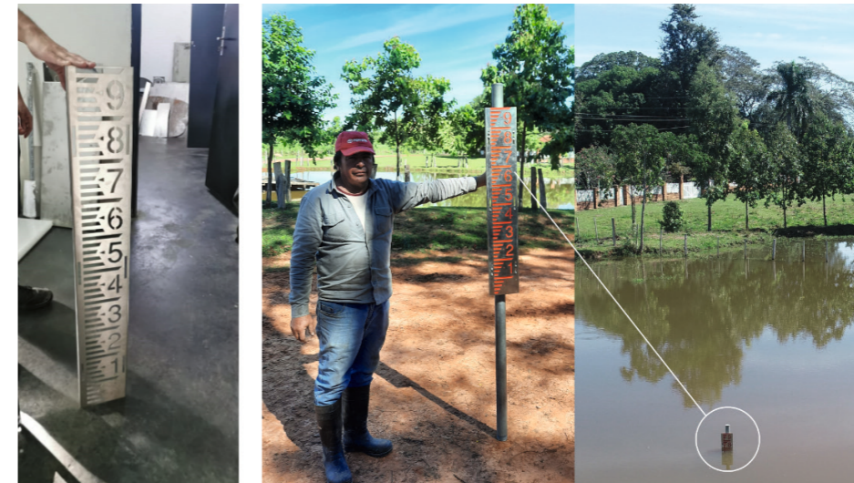
Fig. 2: A Staff gauge in stainless steel fabricated with CNC laser and B Installation of the staff gauge in a water reservoir at a cattle ranch
