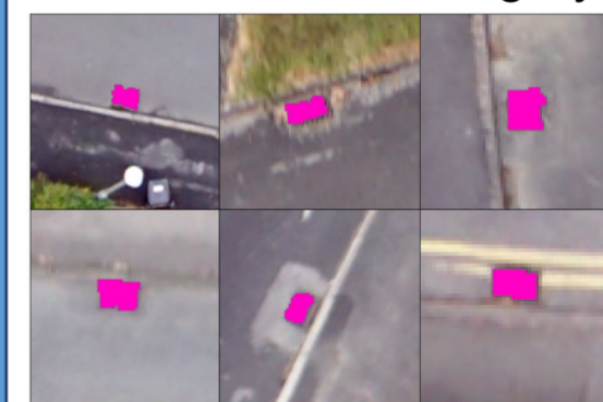
Figure 6. Example of gullies identified using AI algorithms from high-resolution Unmanned Aerial Vehicle imagery
