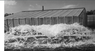
A vertical pump aerator
