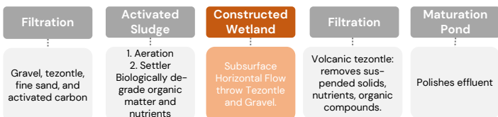
Figure 1. Hybrid System for Biological Treatment for Liquid Waste Generated in Livestock Processes. [1] Own Elaboration.
